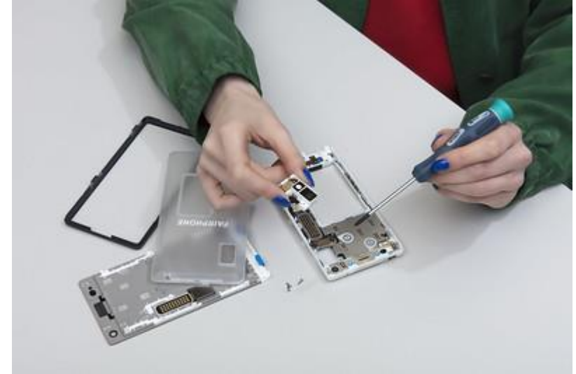
Figure: Fairphone, an example of modular design of electronics, which enables repairing and replacing of certain components https://www.flickr.com/photos/fairphone/28275505528/in/album-72157632717840706/
